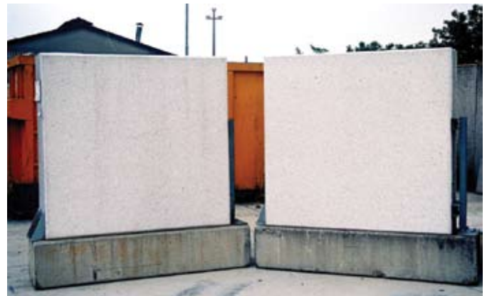
Fig. 1: A demonstration of the cleaning action of photocatalytic cement concrete. The panel on the right contained TX Active
